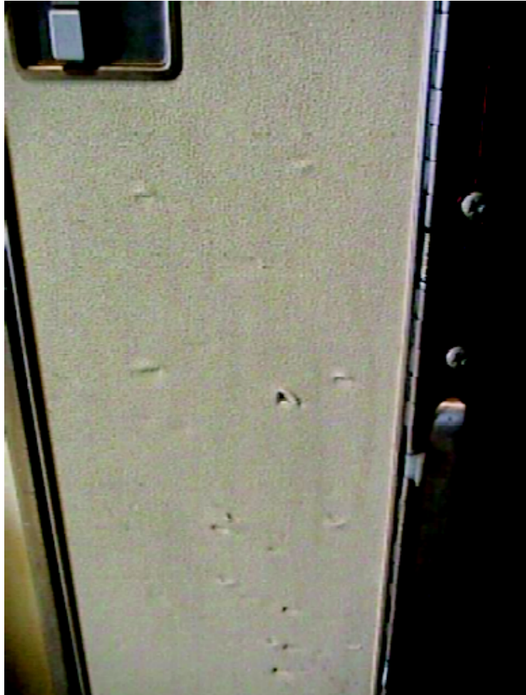
Extensive Damage on Tedlar Figure 6010/GRAPHIC 25-40-53-300-010-A01
